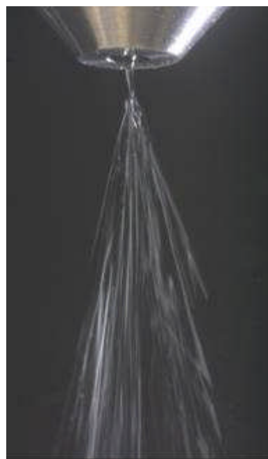
Figure 4. Image of one of the basic two-fluid atomizers operating on medium viscosity alginate (800cp).
