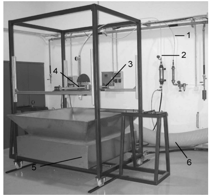
Fig. 3. Photo of the experimental facility: 1- air line, 2- water line, 3- displacement and positioning system, 4- nozzle assembly, 5- container, 6- air extraction tube.
