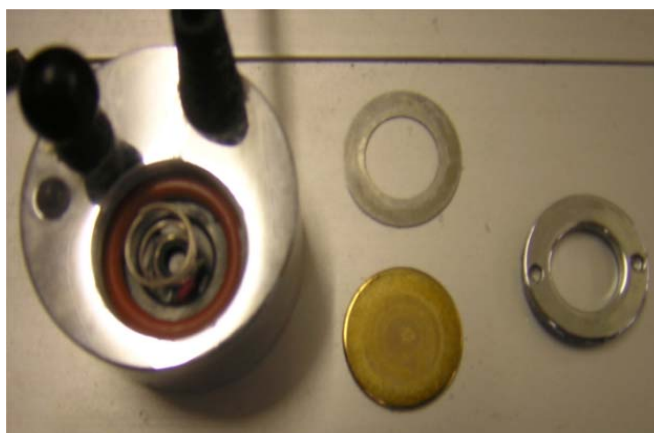
Figure 1 The ultrasonic atomizer and its components; Author, 2005
