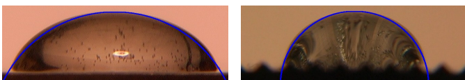
Fig. 8 Deviation from the “circular profile” approximation for two V = 85 \cdot 10^{-9} \text{ m}^3 drops on a smooth (Ot000) and a microfinned (Ot400) surface.
