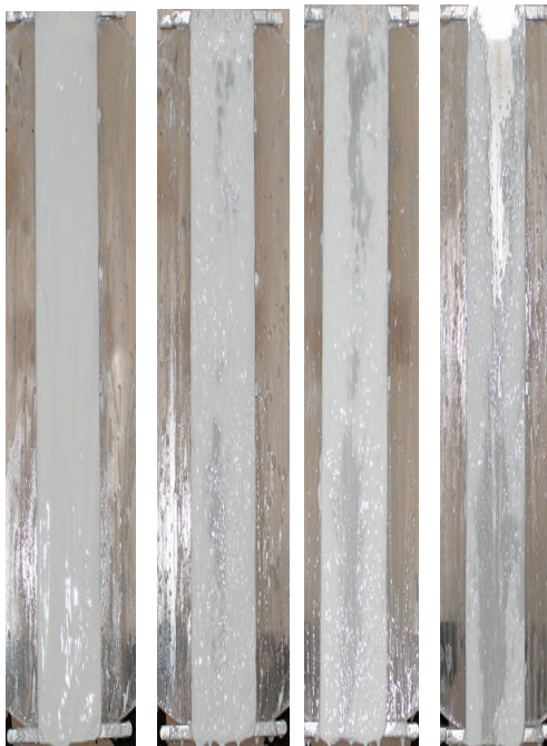
Figure 9: Nozzle B at 5m, 8bar, 38litres/min, 3.4rpm 3 scans.
