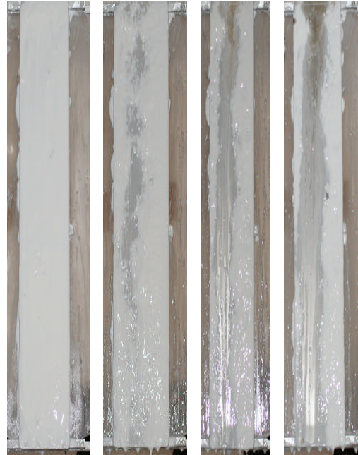
Figure 10: Nozzle E at 5m, 11.2bar, 38litres/min, 3.4rpm 3 scans .
