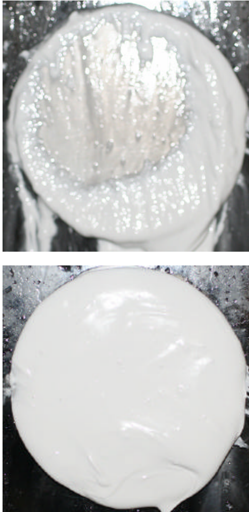
Figure 3: Example of paste coated target before and 1 second after spray impact
