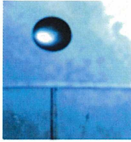
Figure 4. Test Droplet Approaching Surface of a Capillary Block
