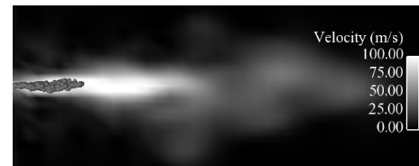
Figure 6. Magnitude of Velocity obtained using linear interpolation of the advection term. Non-physical wiggles can be seen around the injector.
