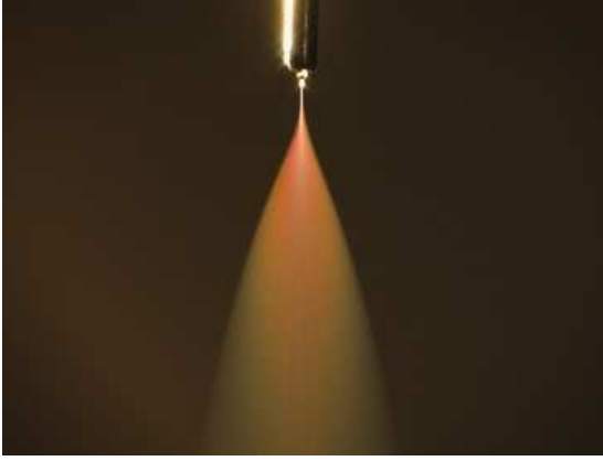
Fig. 3. Cone-jet mode of electro spraying of methanol. Capillary: 0.45 mm o.d., 0.25 mm i.d., flow rate 0.1 ml/h, voltage 8 kV, capillary-substrate distance 30 mm.
