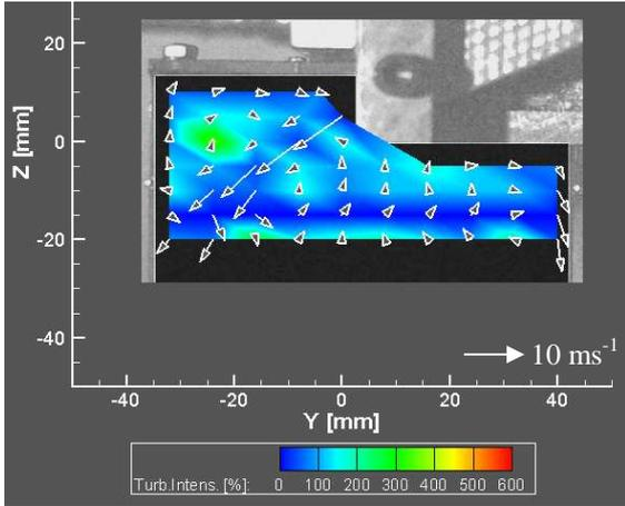
Figure 7: Mean steady flow and turbulence intensity for  $L_v = 9$  mm, fixed air mass flow rate of  $0.01 \text{ kgs}^{-1}$  in TP2
