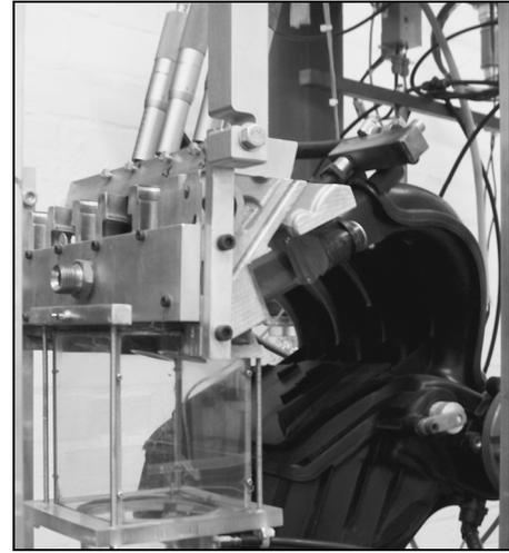
**Figure 1:** Modified cylinder head and steady-state flow rig assembly
