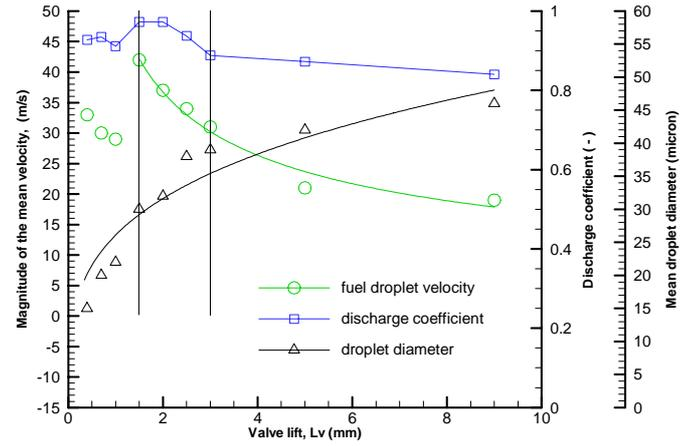
**Figure 13:** Variation in peak mean steady flow velocity and droplet diameter versus valve-lift for fixed flow conditions.
