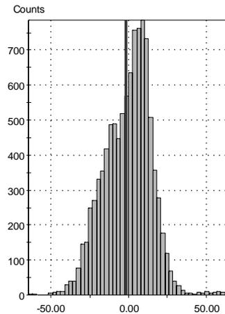
(a) Axial droplet velocity component ( $\text{ms}^{-1}$ ) at 10 mm below the gas face
