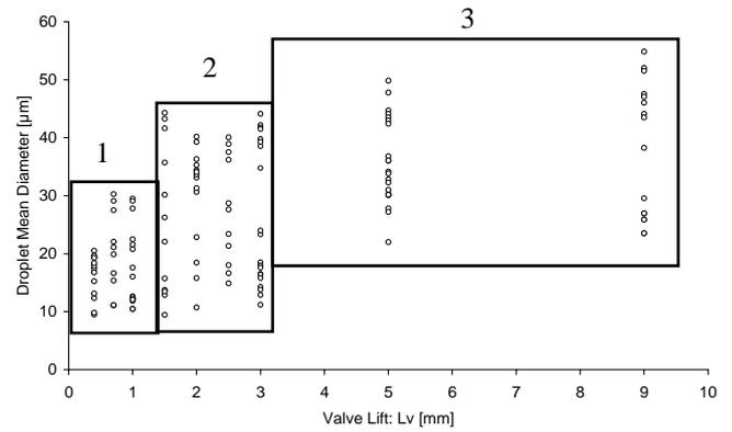
**Figure 11:** Range of mean droplet diameters across all measuring locations against valve lift for tumble plane TP2
