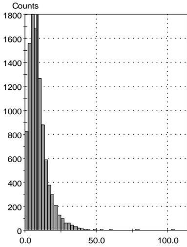
(c) Droplet diameter ( $\mu\text{m}$ ) at 10 mm below the gas face
