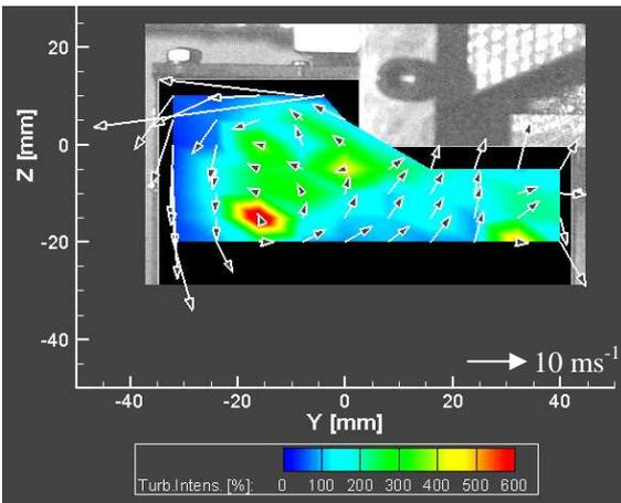
Figure 8: Mean steady flow and turbulence intensity for  $L_v = 0.4$  mm, fixed air mass flow rate of  $0.01 \text{ kgs}^{-1}$  in TP2
