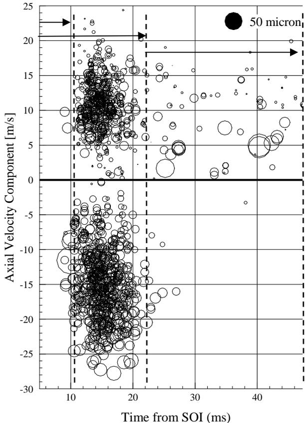
**Figure 12:** Time series of droplet axial velocity after SOI for fixed pressure conditions and  $L_v=0.4 \text{ mm}$
