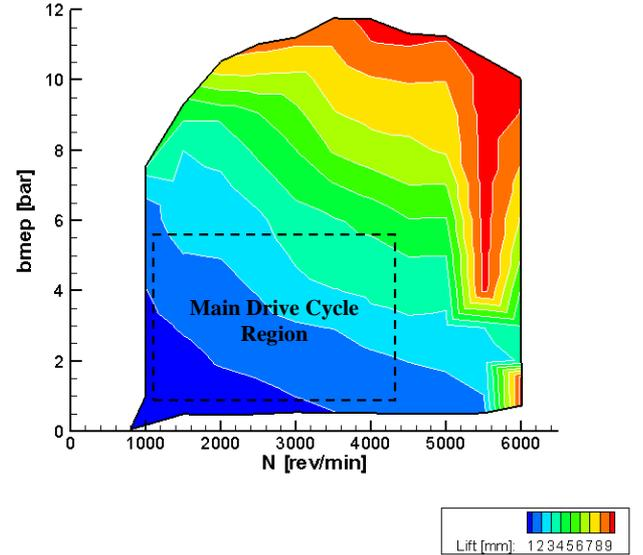
Figure 3: Variation in peak intake valve lift with engine speed and load for the BMW Valvetronic engine.
