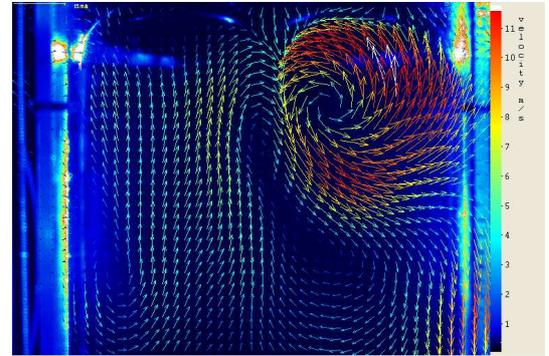
**Figure 6:** Mean air motion in cross-tumble plane, CT1 for  $L_v = 2.5$  mm, fixed pressure drop of 40 mbar
