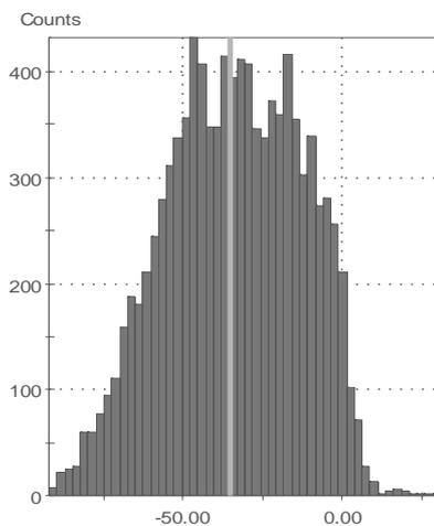
(b) Radial droplet velocity ( $\text{ms}^{-1}$ ) component at 10 mm below the gas face
