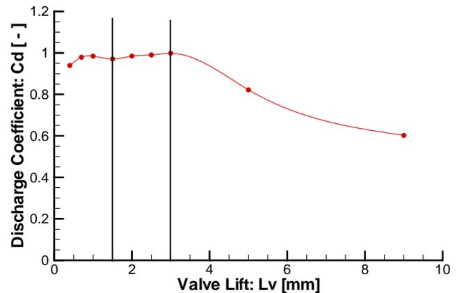
Figure 4: Variation in discharge coefficient with valve lift for a fixed pressure drop of 40 mbar.
