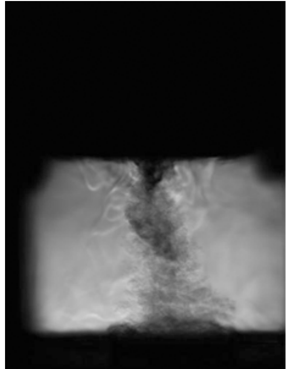
Figure 11: Front view. Schlieren images of the sprays from the nozzle with 10^\circ angular spacing between the sprays, 1.5 ms after energizing the injector and 900 bar. Flat wall.
