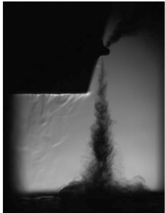
Figure 12: Side view. Schlieren images of the spray from the conventional three-hole nozzle, 1.5 ms after energizing the injector and 900 bar. Flat wall.
