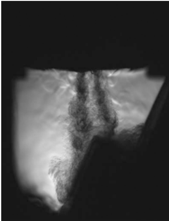
Figure 7: Schlieren image of the sprays from the nozzle with 20° angular spacing between the sprays, 1.5 ms after energizing the injector and 900 bar. Slant divided wall.
