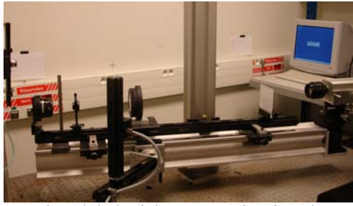
Figure 6: the Global rainbow setup developed at Rouen.
