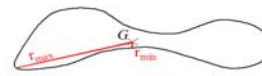
Figure 5: Uniformity ( \eta ): difference between the maximum and minimum radius over perfect disk radius
