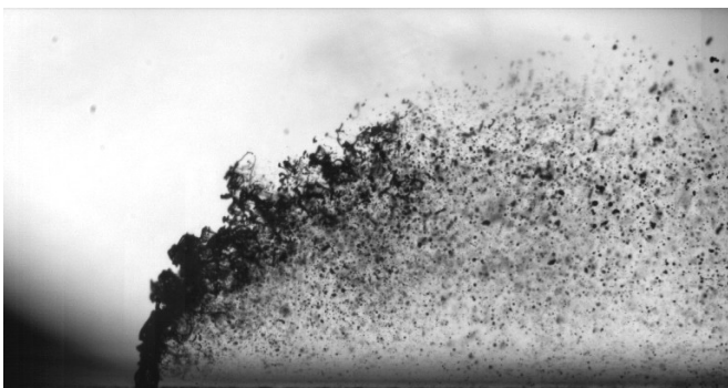
Fig. 3 : Single shadowgraph image of the kerosene spray entering an oncoming flow of U_\infty = 50 m/s from the left. LED illumination pulse was 230 ns. The field of view is 11 mm wide (Flow parameters: D=0.3 mm, U_\infty=50 m/s, p=4 bar).
