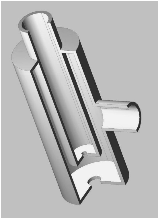
Figure 2. Investigated nozzles construction
