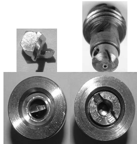
Figure 4. TG2 (left) and TG0.7 (right) internal geometry.
