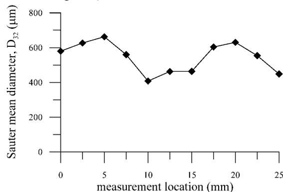
Figure 1:  $D_{32}$  versus axial measurement location [1].
