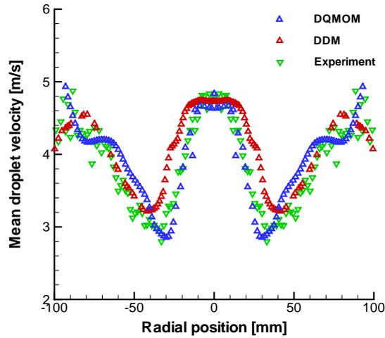
**Figure 5.** Experimental and numerical profiles of the mean droplet velocity at the cross section of 0.12 m distance from the nozzle exit
