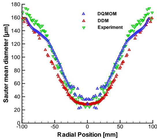
**Figure 1.** Experimental and numerical profiles of the Sauter mean diameter at the cross section of 0.12 m distance from the nozzle exit
