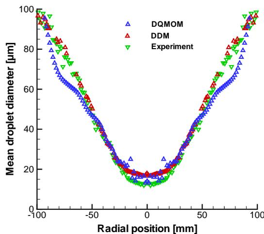
**Figure 3.** Experimental and numerical profiles of the mean droplet diameter at the cross section of 0.12 m distance from the nozzle exit
