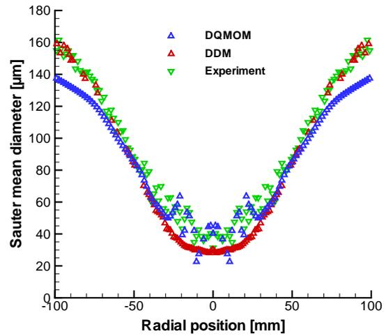
**Figure 2.** Experimental and numerical profiles of the Sauter mean diameter at the cross section of 0.16 m distance from the nozzle exit
