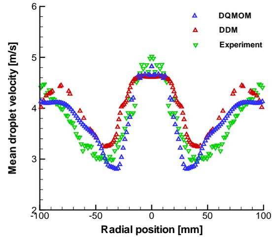
**Figure 6.** Experimental and numerical profiles of the mean droplet velocity at the cross section of 0.16 m distance from the nozzle exit
