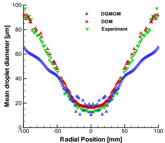
**Figure 4.** Experimental and numerical profiles of the mean droplet diameter at the cross section of 0.16 m distance from the nozzle exit
