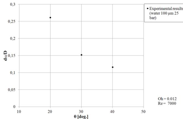
Fig. 9: Dependence of SMD on impingement angle. water (Oh = 0.012, Re = 7000)
