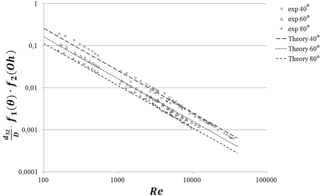
Fig. 12: Comparison of experimental data with theoretical prediction.
