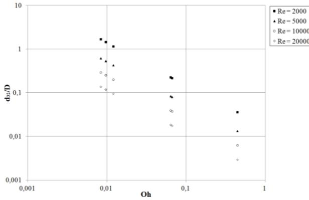
Fig. 6: Dependence of SMD on Oh with impingement angle 40°.
