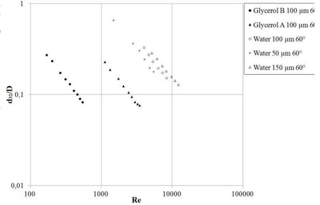
**Fig. 4:** Dependence of SMD on Re with impingement angle 60°. Glycerol A ( $\mu = 0.0058$  Pa s) Glycerol B ( $\mu = 0.039$  Pa s)
