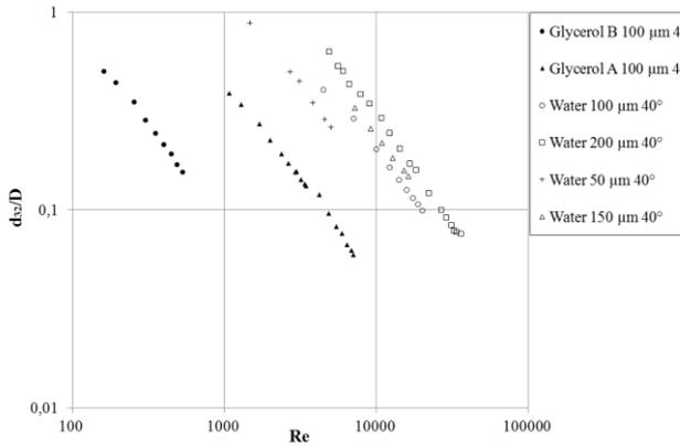
**Fig. 3:** Dependence of SMD on Re with impingement angle 40°. Glycerol A ( $\mu = 0.0058$  Pa s) Glycerol B ( $\mu = 0.039$  Pa s)
