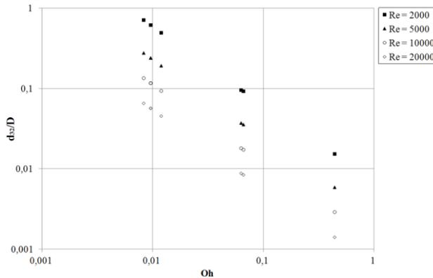
Fig. 8: Dependence of SMD on Oh with impingement angle 80°.
