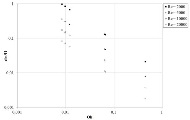
Fig. 7: Dependence of SMD on Oh with impingement angle 60°.
