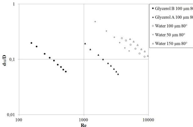
**Fig. 5:** Dependence of SMD on Re with impingement angle 80°. Glycerol A ( $\mu = 0.0058$  Pa s) Glycerol B ( $\mu = 0.039$  Pa s)
