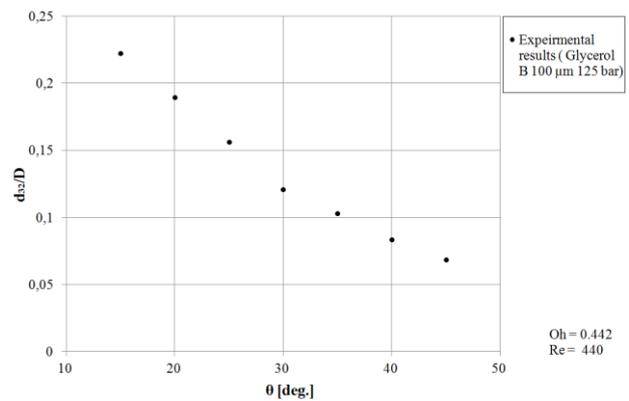
Fig. 10: Dependence of SMD on impingement angle. water – glycerol solution B (Oh = 0.442, Re = 440)
