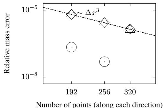
Figure 2: Relative mass error for sphere deformation test case (backward: triangles, forward: diamonds, trapezoidal: circles).
