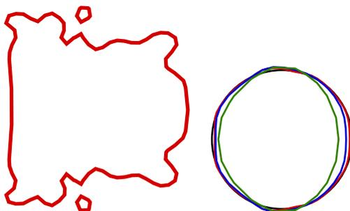
Figure 3: High density ratio ( $10^9$ ) drop ( $32 \times 32$ : green,  $64 \times 64$ : blue,  $128 \times 128$ : red): non-conservative scheme at time  $t/T = 0.05$  and conservative scheme at time  $t/T = 1.0$ .
