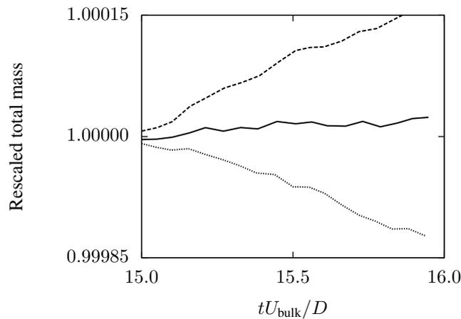
Figure 5: Relative mass error in diesel jet (backward: dashed line, forward: dotted line, trapezoidal: solid line).
