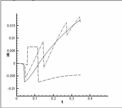
Figure 3. Evolution of the Lateral Displacement of the position of Maximum Axial Deformation relative to the Droplet Origin for 3 Cases :  $\eta_d/\eta_g = 16$ ,  $\rho_d/\rho_g = 550$ , (i) Full Line –  $We = 15$ ,  $Re = 1000$ , (ii) Dash Line –  $We = 1$ ,  $Re = 1000$ , (iii) Dot-Dash line –  $We = 15$ ,  $Re = 100$
