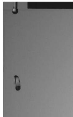
Figure 1. High-speed Image of Droplet Deformation Prior to Breakup in an Air-Flow (left-to-right)
