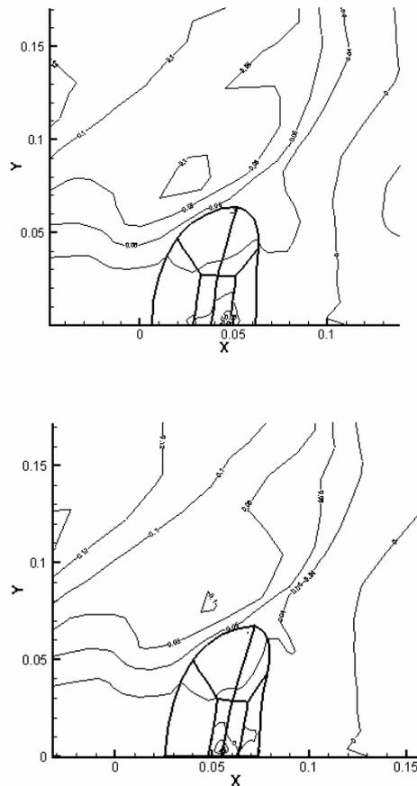
Figure 2. Predicted Droplet Deformation, Translation and Velocity Magnitude Contours - Benchmark Newtonian Problem.  $T = 0.03, 0.15, 0.21, 0.27, 0.33$
