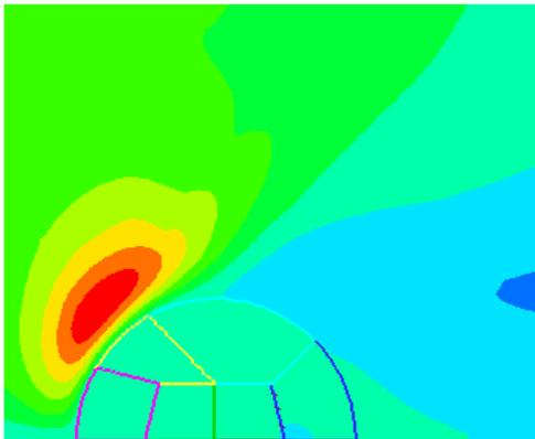
Figure 4. Droplet Deformation and Velocity Magnitude Contours of a Liquid Droplet in a Flow at 10x the Viscosity Ratio compared with Benchmark Case, all other parameters constant
