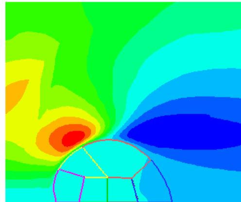
Figure 5. Droplet Deformation and Contours of Velocity Magnitude for a Blood Droplet represented by the Shear-thinning Model of Cross (10)
