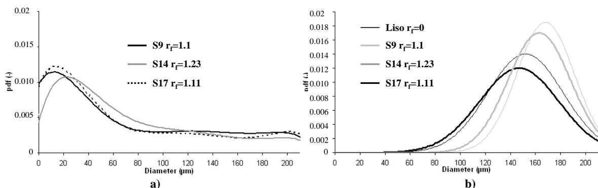
PDF of the secondary droplet size resulting from the impact of a monosize stream of ethanol droplets ( $D_0=180 \mu\text{m}$ ,  $U_0=3.2 \text{ m/s}$ ) over the micro-textured surfaces (Liso to S17) within: **a)** nucleate boiling regime ( $T_{w,0}=130^\circ\text{C}$ ) **b)** film boiling regime ( $T_{w,0}=200^\circ\text{C}$ ). PDA measurements performed at  $r=1.2 \text{ mm}$ ,  $z=1.2 \text{ mm}$ .
