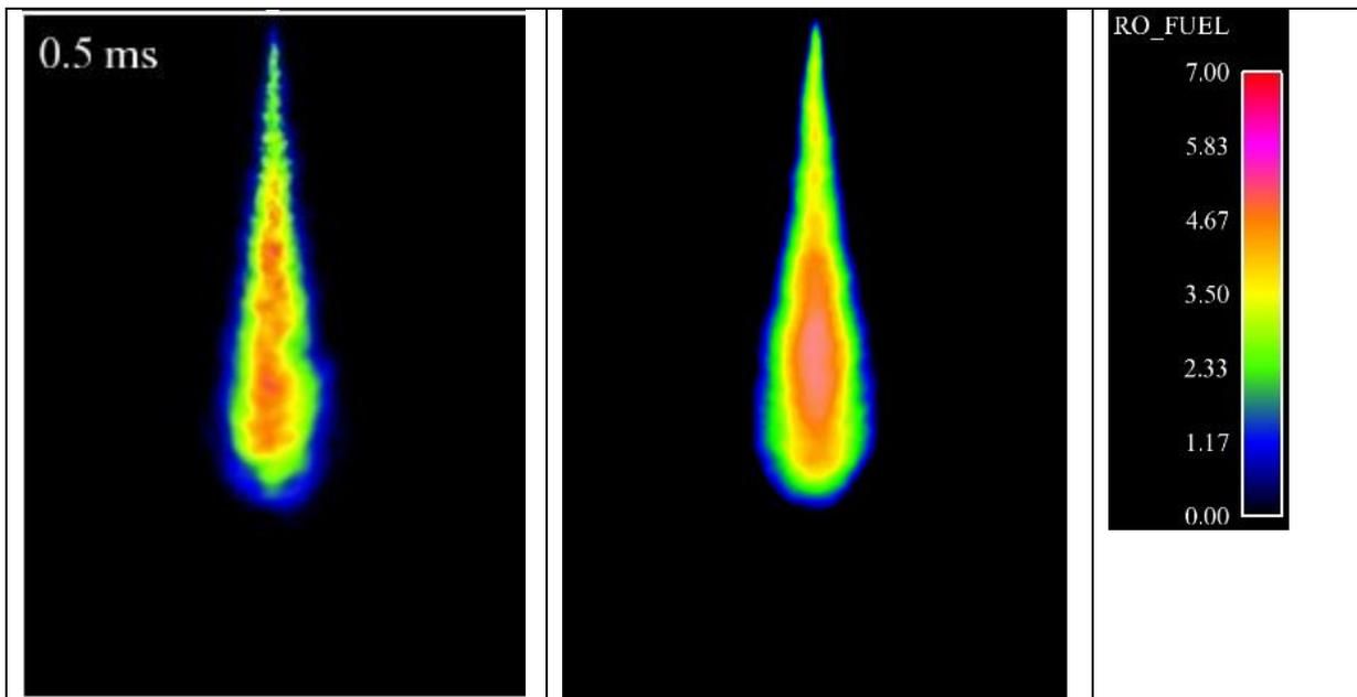
**Figure 2** Averaged results of T9P12 case 1. Quantitative comparison of the experimental (right) and LES (left) averaged fuel mass density results at 0.5 ms. The same color pallet of the fuel mass density is used for the numerical and experimental results (RO\_FUEL in kg/m<sup>3</sup>).
