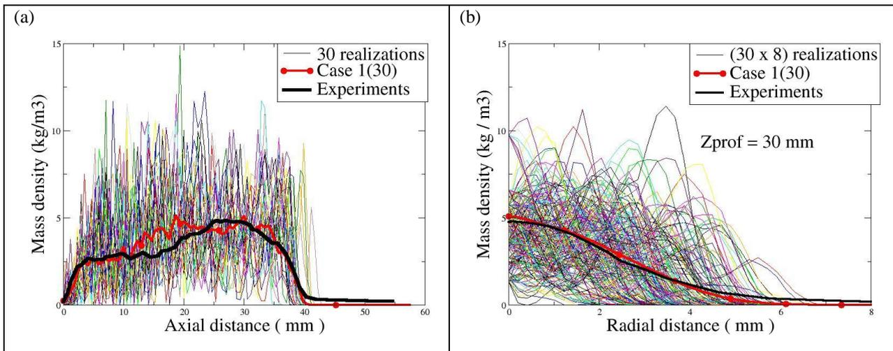
**Figure 1** Results of T9P12 case 1:  $P_{inj} = 120$  MPa,  $T_{gas} = 900$  K and  $P_{gas} = 6.7$  MPa.. Comparison of the experimental and LES axial (a) radial (b) profiles of the fuel mass density at axial location ( $Z_{prof}=30$  mm) from the nozzle exit and at time  $t=0.5$  ms. The red curve with solid circles is the average of ( $30 \times 8 = 240$ ) LES profiles depicted by thin lines. The experimental profiles are the results of the averaging of 50 injections.
