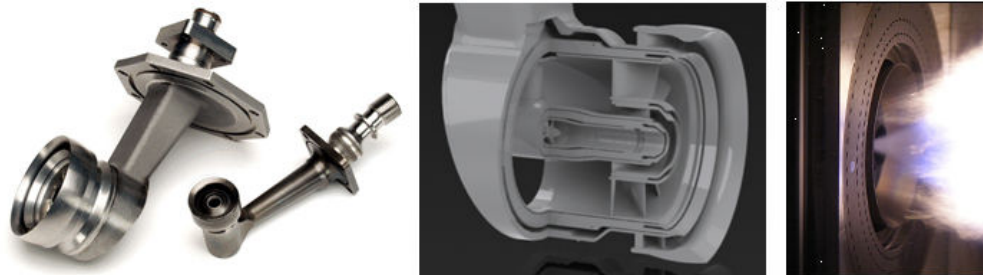
Fig. 2 Rolls-Royce Internally Staged Lean Direct Injection Fuel Spray Nozzle
