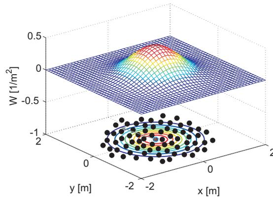
**Figure 1.** Kernel function for interpolation on center particle (blue)
