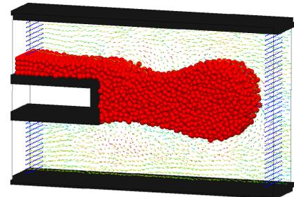
**Figure 9.** Three-dimensional film disintegration at atomizer edge
