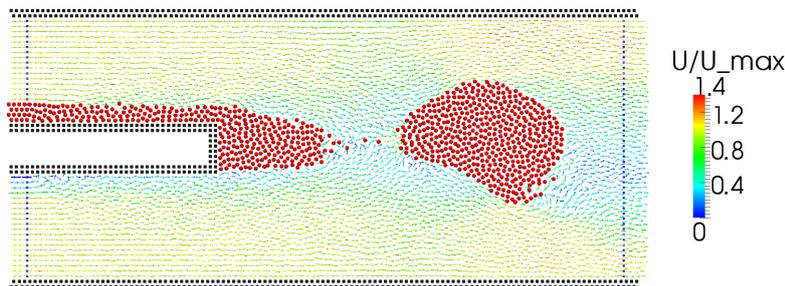
**Figure 8.** Film disintegration and shear-off of a liquid ligament
