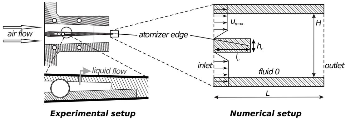
**Figure 7.** Experimental and numerical setup for film disintegration investigations
