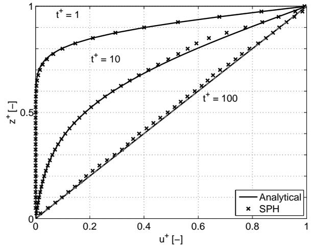
**Figure 2.** Numerical setup for Couette flow simulations **Figure 3.** Transient velocity profiles of Couette flow for  $Re = 100$
