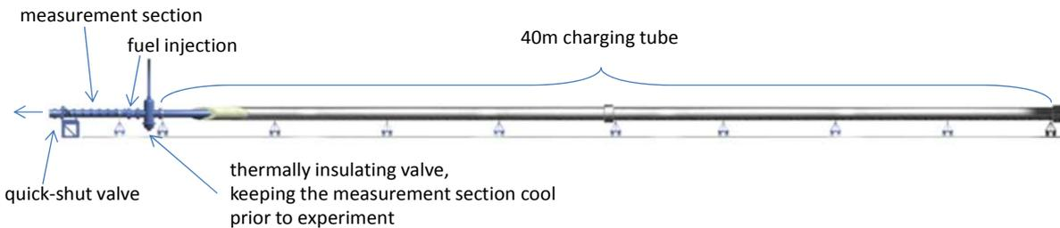
**Figure 1** Hot blowdown windtunnel
