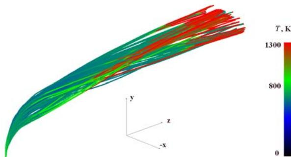
**Figure 4** Spraylet trajectories with color changing into red where hot flame occurs
