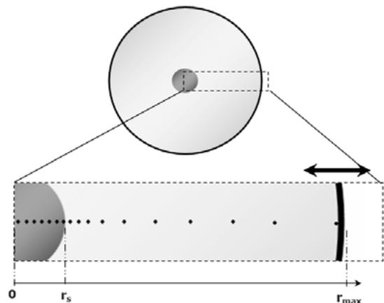
**Figure 3** Schematic of the numerical grid and the boundaries of the spraylet model
