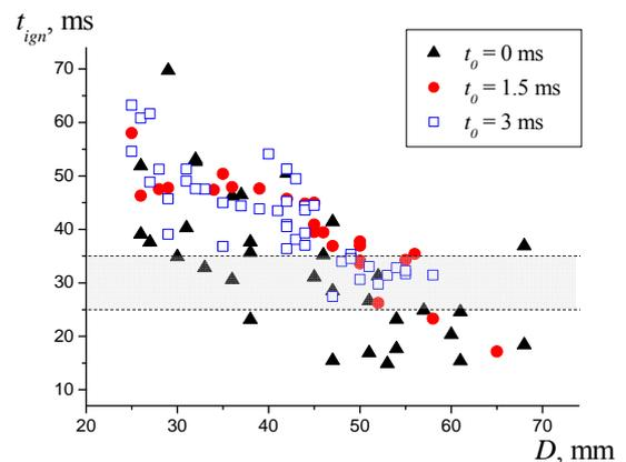
**Figure 5** Total induction time of experiments (gray area) and numerical results (symbols) showing the effect of initial droplet size and the position in the spray (black triangles = front of the spray; red dots and blue squares = developed spray)
