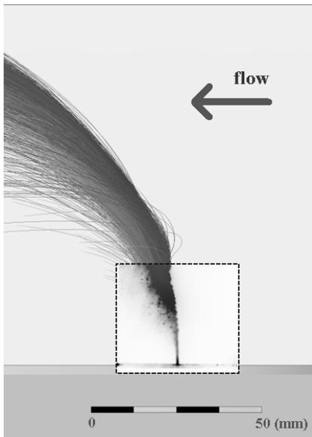
**Figure 2** Jet in cross flow injection. Comparison between simulation and experiment
