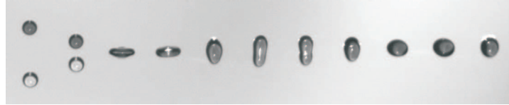
Figure 3. Full encapsulation of a 50 % glycerol solution drop by SO M20. The relative velocity of the drops at the impact is 3.88 m/s.
