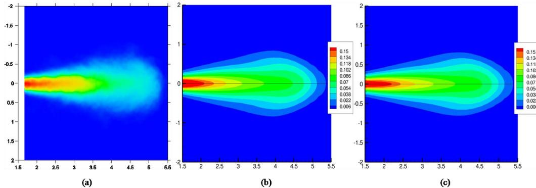
**Figure 1.** Measured (a), and computed vapor fraction contours at 1.13 ms ASI; (b) is with vapor jet and (c) is with liquid spray. Color legend identifies values of vapor fraction [7].
