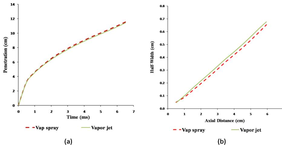
**Figure 2.** (a) Penetrations and (b) half-widths of the computed vapor jet and spray [9].
