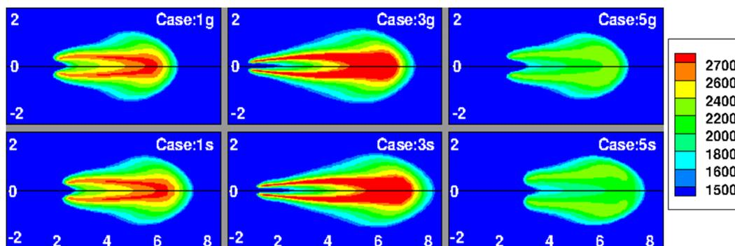
**Figure 3.** Computed temperature contours for spray and vapor jets at 2.5 ms ASI.
