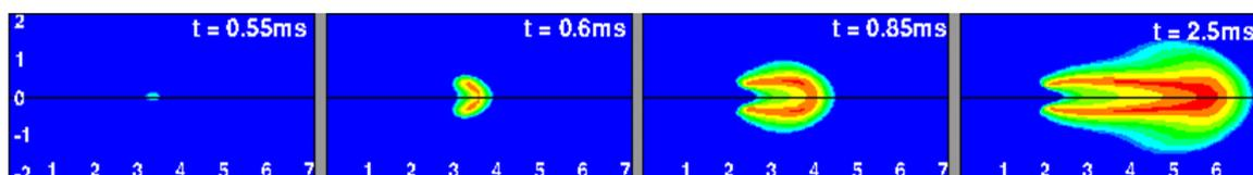
**Figure 4.** Transient development of temperature contours for the vapor jet.
