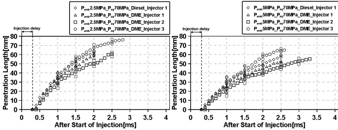
Figure 11 Spray development length at  $P_{amb} : 2.5$ (left) and 5 MPa (right),  $P_{inj} : 70$  MPa
