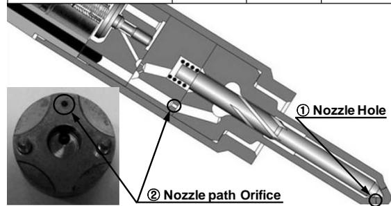
Figure 3 Specifications of test injectors
