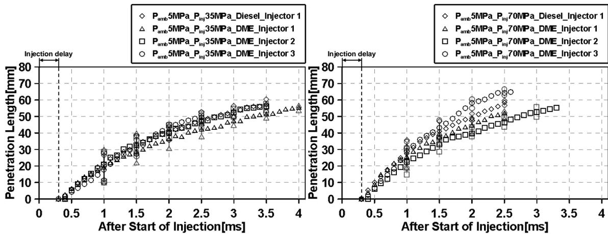
Figure 10 Spray development length at  $P_{amb} : 5 \text{ MPa}$ ,  $P_{inj} : 35$  (left),  $70 \text{ MPa}$  (right)
