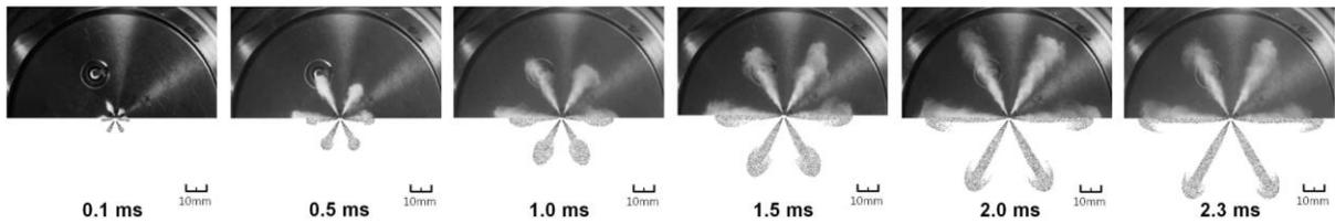
**Figure 14 Comparison between experiment and simulation of the DME spray at  $P_{amb} : 5 \text{ MPa}$ ,  $P_{inj} : 35 \text{ MPa}$**
