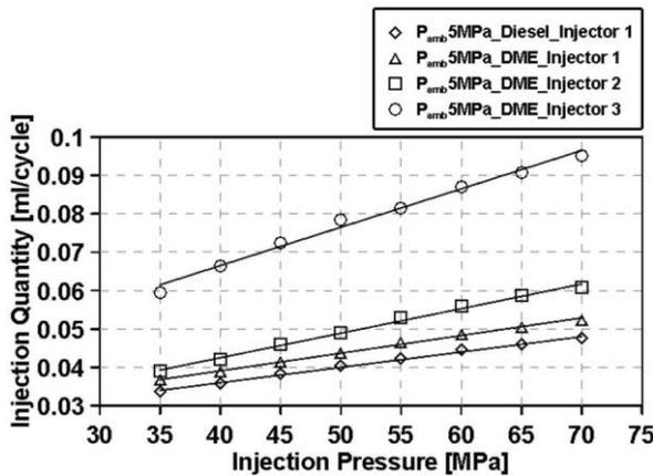
Figure 7 Single injection quantity [ml/cycle]
