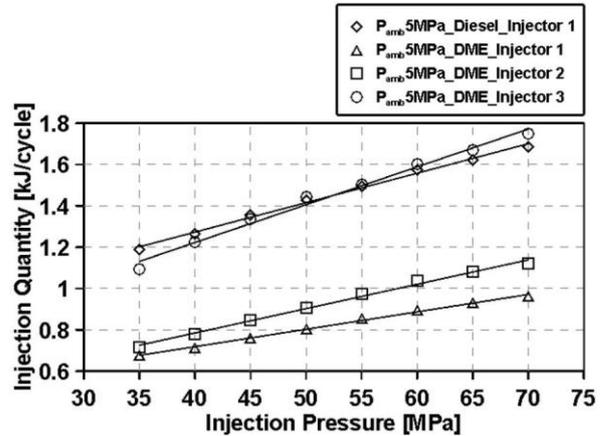
Figure 8 Single injection quantity [kJ/cycle]
