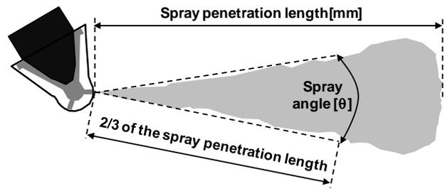
Figure 5 Spray shape measurement elements
