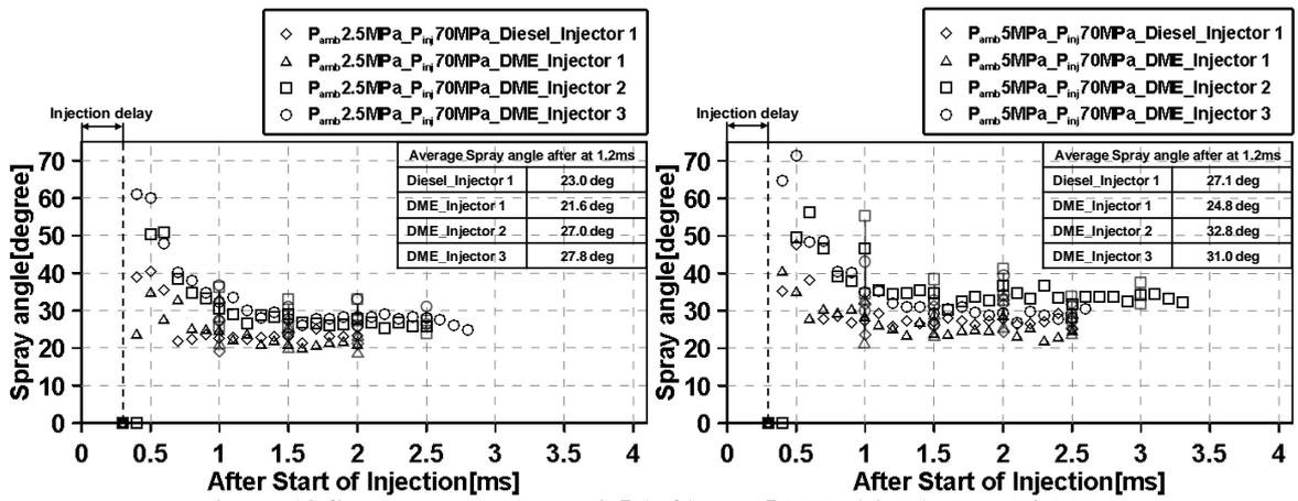
Figure 13 Spray angle at  $P_{amb} : 2.5$  (left) and 5 MPa (right),  $P_{inj} : 70$  MPa
