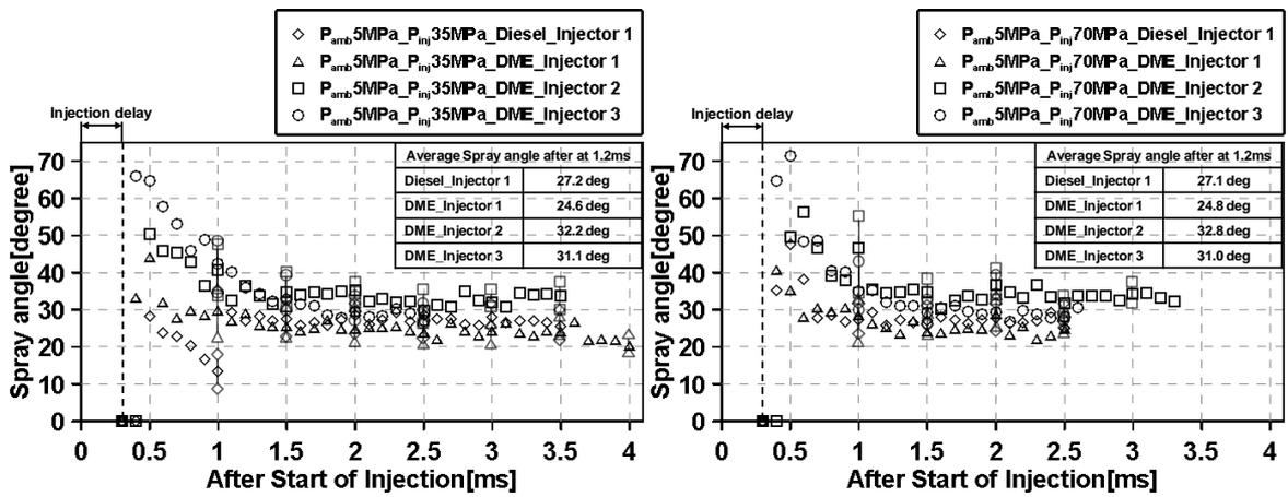
Figure 12 Spray angle at  $P_{amb} : 5$  MPa,  $P_{inj} : 35$  (left) and 70 MPa (right)
