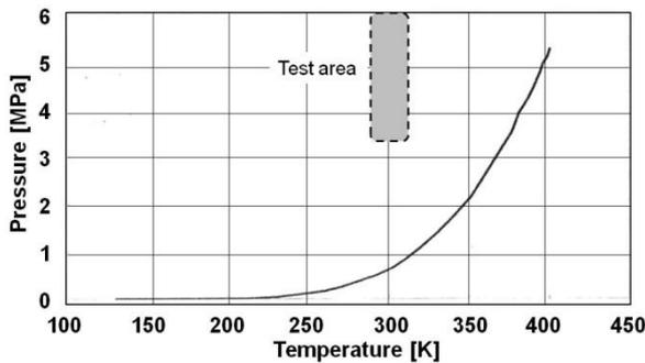
Figure 2 Vapor pressure curve of DME
