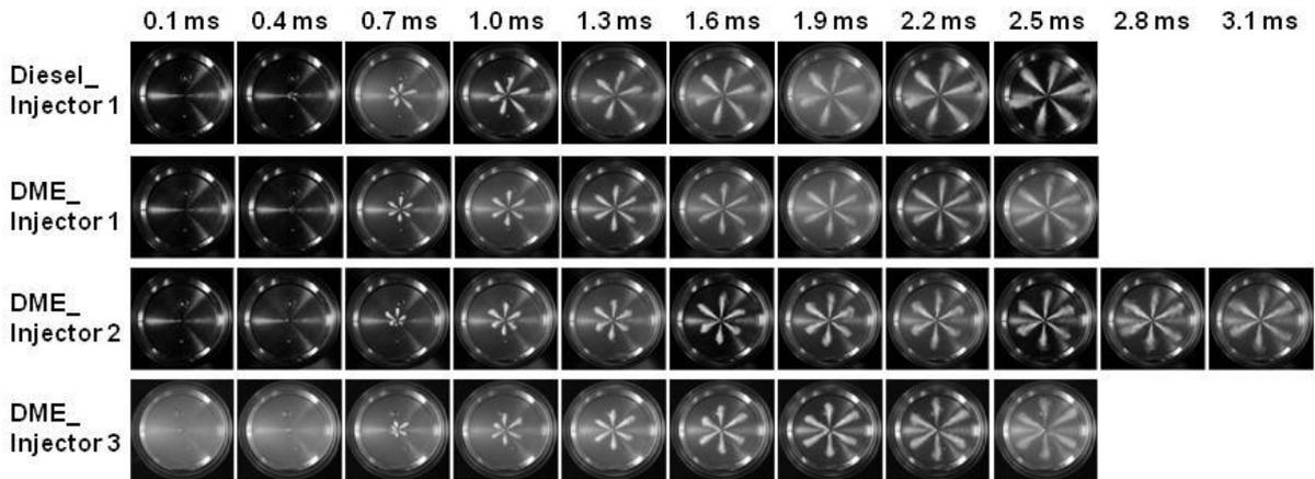
Figure 9 Spray development process at  $P_{amb} : 5 \text{ MPa}$ ,  $P_{inj} : 70 \text{ MPa}$
