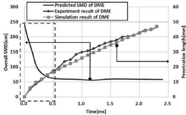
**Figure 15 Penetration length of DME and predicted SMD**
