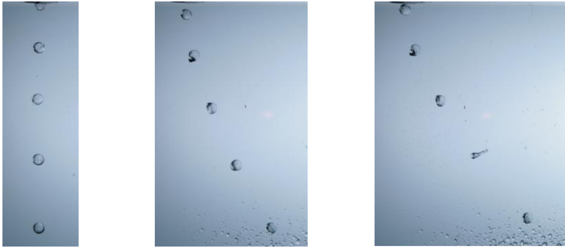
(a) u_a=0, We_b=0, Re=0 (b) u_a= 8.06 \text{ m/s}, We_b= 1.12, Re = 36.8 \times 10^3 (c) u_a= 9.87 \text{ m/s}, We_b= 1.68, Re = 45.1 \times 10^3
