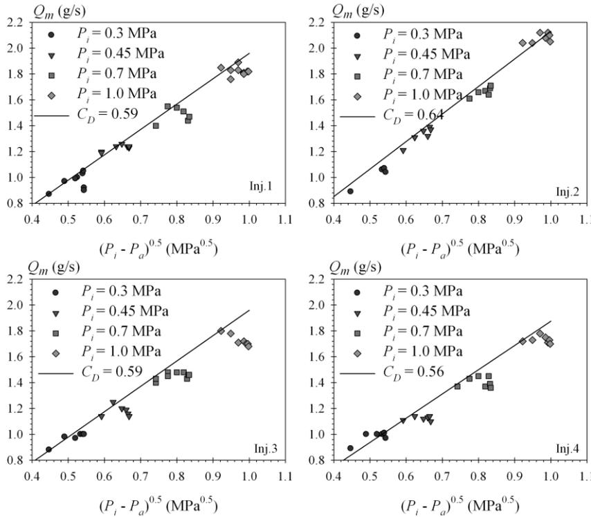
**Figure 2** Fully-open stage mass flow rate as a function of the injection and ambient pressures  $P_i$  and  $P_a$  (the line illustrates the dependence with the discharge coefficient measured under atmospheric pressure  $P_a = 0.1$  MPa)
