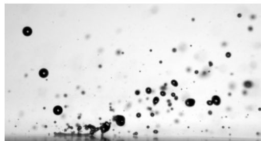
Figure 3 Splashing of water droplets ( D_d=118 \mu\text{m} , We_n=107.4 , V=8.645 \text{ m/s} , f_{inj}=16\ 400 \text{ Hz} )
