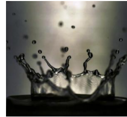
Figure 2. The splashing event captured at 15 ms after impact for We = 810 .
