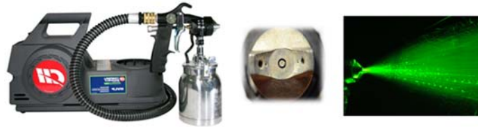
Figure 1 HVLP spray system and spray image
