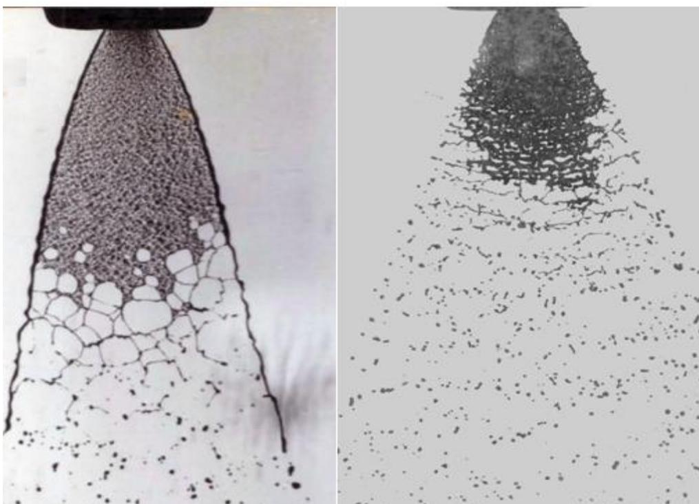
**Fig. 1 : Photographs of sheets containing Attapulgitic particles (left) and Glass particles (right) undergoing break-up. The Nozzle is Titan 521, Sheet velocities are ca. 22m/s**
