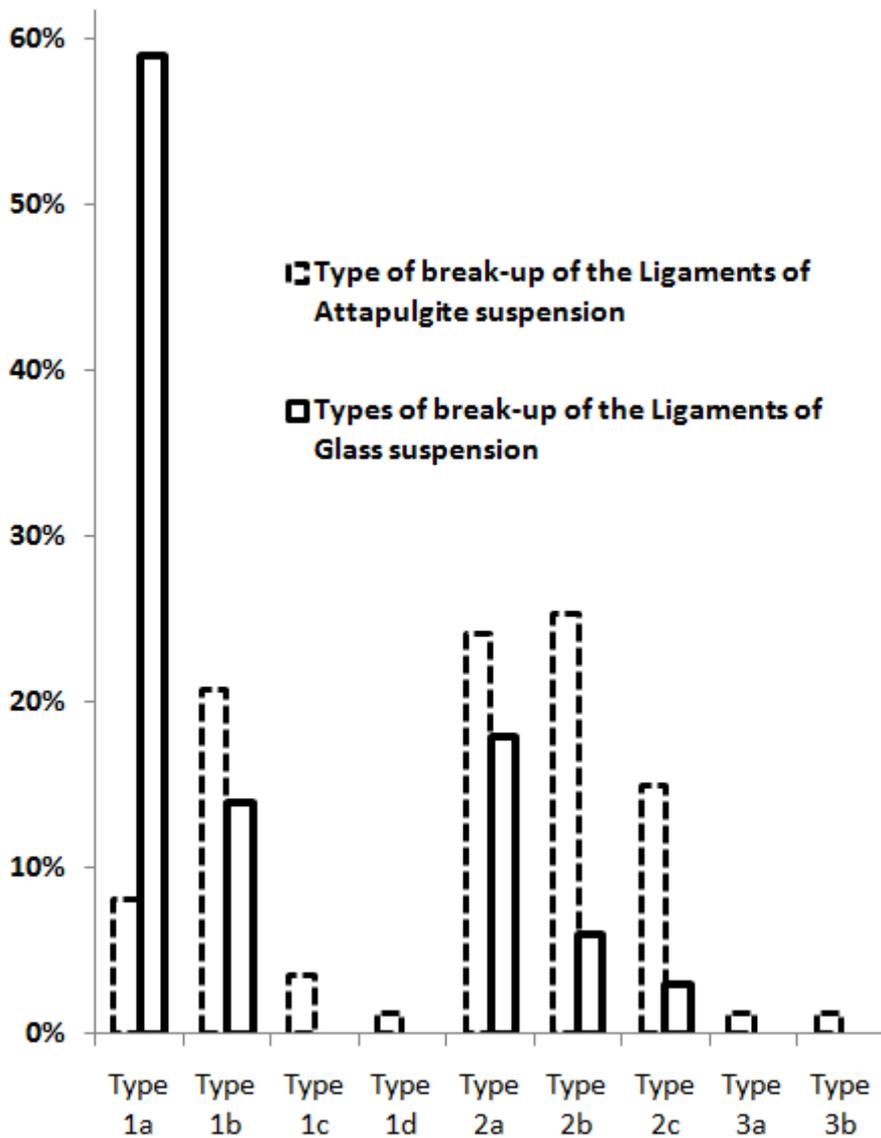
**Fig. 4: Types of Break-up of network formed by sheets of suspensions of Glass and Attapulgit (Nozzle Titan 521 & 943, Velocity 22m/s)**
