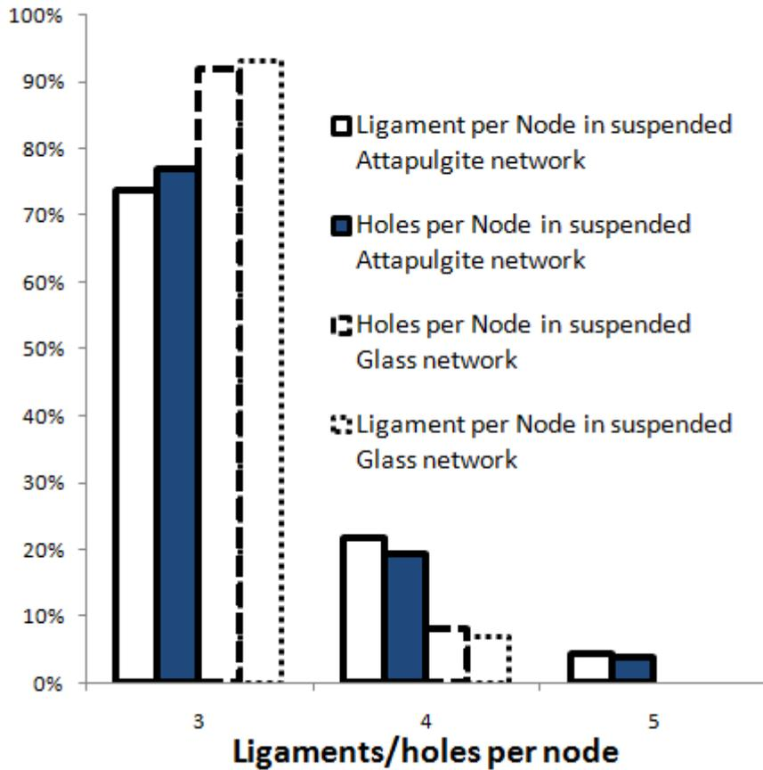
Fig. 3: Bar chart of the Distribution of Ligaments per node and Holes per node in the network formed by sheets Glass and Attapulгите Suspensions
