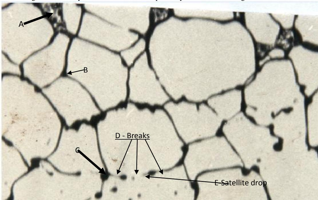
**Figure 2: High magnification photograph (X 22.6) of network formed by suspension of Attapulgate clay showing fracture of ligaments.**
