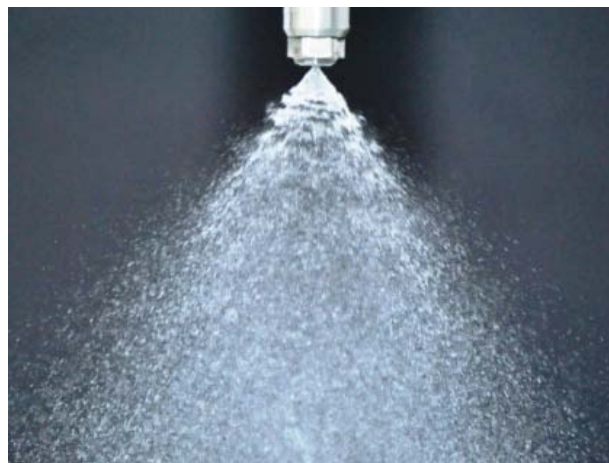
Figure 3: Spray Visualization during the Experiment of Diesel Spray at 8Bar
