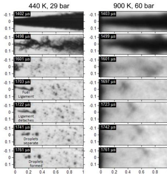
Figure 6: Visualization of liquid n-dodecane jets injected at reference conditions where the ambient gas is  $p_1 = 29 \text{ bar}$ ,  $T_1 = 440 \text{ K}$  and  $p_2 = 60 \text{ bar}$ ,  $T_2 = 900 \text{ K}$ . At low temperatures there is evidence of drops and ligaments. At high temperatures there is no evidence of drops or ligaments.
