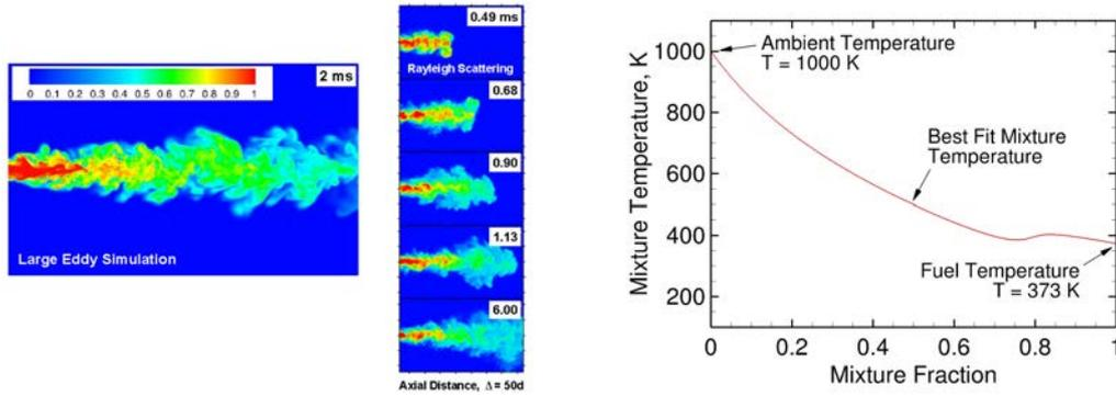
Figure 3: Comparison of mixture fraction predictions from LES (left) with measured Rayleigh images (center). Corresponding best fit mapping of temperature as a function of mixture fraction for the time evolving field (right).
