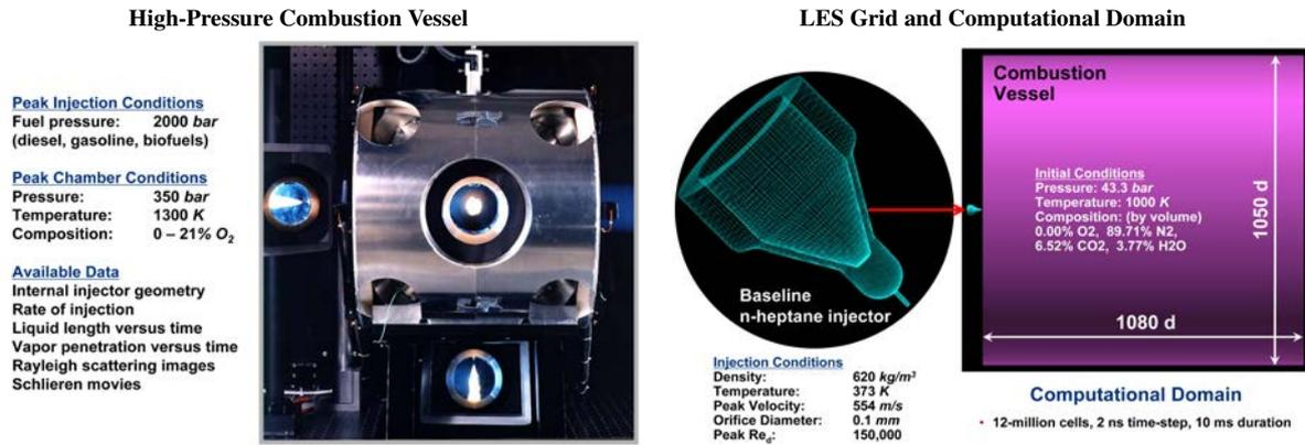
Figure 1: Photograph of the Sandia high-pressure combustion vessel (left) and computational domain used for LES (right). The injector is mounted at the head-end of the vessel, as indicated by the red arrow. The grid and operating conditions identically match the experiment. Conditions listed correspond to the Baseline n-Heptane experiment.
