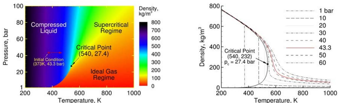
Figure 2: Thermodynamic characteristics of n-heptane showing key regimes and its initial state when injected into the combustion vessel. The jet enters as a compressed liquid and is heated at supercritical pressure.
