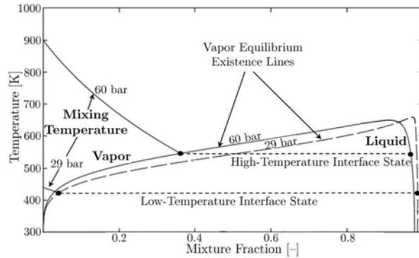
Figure 7: Mixing lines obtained from detailed analysis of the multicomponent mixture states (such as in Fig. 5) combined with VLE theory facilitate application of the LG model. The intersection of respective curves on the vapor side provide the baseline boundary conditions required to reconstruct the multicomponent interfaces.
