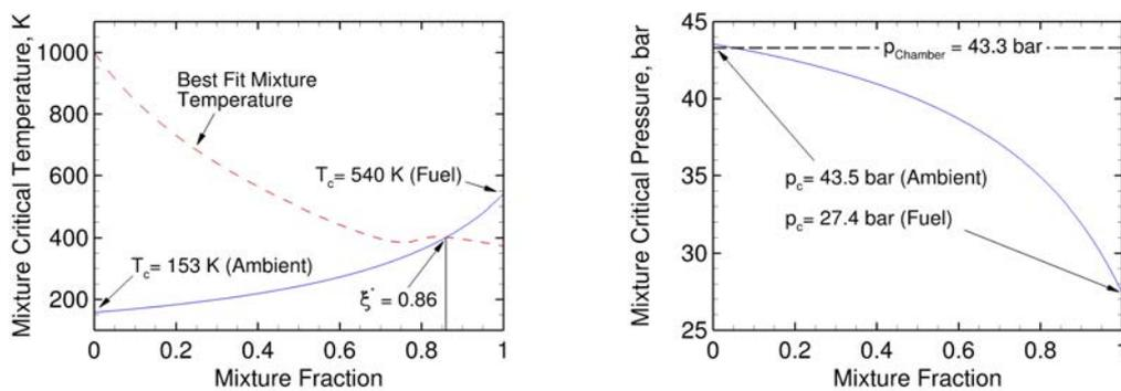
Figure 4: Mixture critical temperature and pressure of the time evolving field as a function of mixture fraction.
