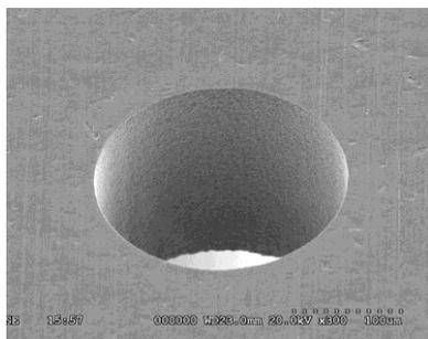
**Figure 1** 200  $\mu\text{m}$  diameter fuel injector spray hole drilled in 250  $\mu\text{m}$  thick stainless steel in 1.3 seconds using femtosecond laser trepanning.
