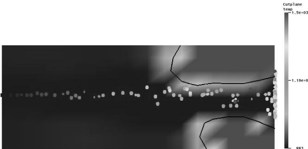
Figure 9. Temperature in a vertical plane passing through the spray axis at t=0.6 ms. Case 2
