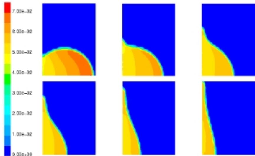
Figure 7. A quarter of a droplet of the non-Newtonian fluid moves to the left towards the origin and collides with its mirror image, realized by a mirror plane on the left. The viscosity \mu (in Pas) at different stages of the collision is visualized in a contour plot.
